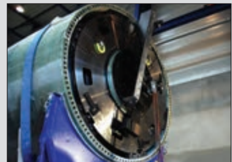
▲ Orbital milling machines for wind turbine manufacture.
