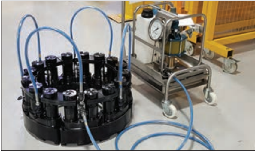
▲ Multi Stud Tensioning Set-Up.
