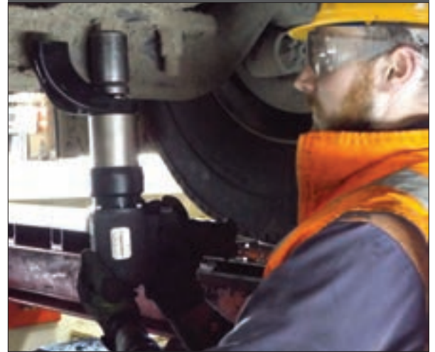
▲ Safe and Quiet Axle Correction with a Pneumatic Torque Wrench.
